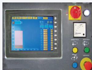
PLC control system with 500 SETS memory capacity
