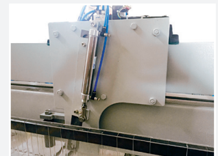
Pneumatic side alignment device for cross cuts (front side)
