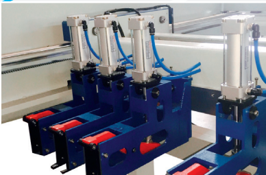
Positioning pusher with grippers (Pneumatic clamp)
