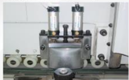
立轴加装气压式上下导板 Moulding unit with pneumatic top pressure pad+bottom support (Chrom plated)
