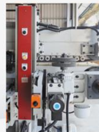
碟型砂光带补偿 Disc sanding unit Motor : 2HP ,Spindle : 1"x 4" with vibration motor with auto. compensation
