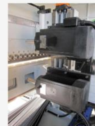
上下鉋 Top and bottom milling unit 7.5HP (special 10HP 15HP) Spindle speed:3000/6000 rpm (50/100HZ) Spindle dimension:Ø40 x 120 mm (L)
