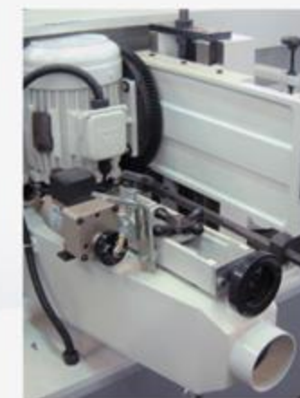
海绵轮砂带座 Sponge sanding unit Motor : 2HP Sanding belt size : 4" x 42" Sponge roller : 7" x 4"
