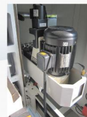
Belt sanding unit Sanding motor: 2HP Sanding belt size: 4" x 60" / 78" / 98" Vibration power: 25w x 1/36
