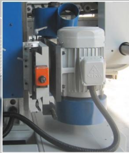
Moulding unit (R) 5HP (option 7.5HP) Spindle speed: 6000 RPM Spindle size: Ø40 MM x 82MM Space required: 450 MM
